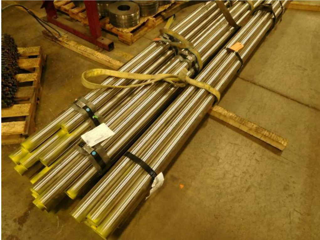
Figure D-1 – Stainless steel bar stock prior to threading.
