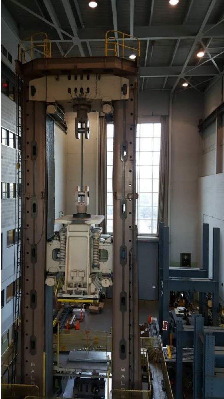
Figure E-15 – Overall view of the tension test set-up in the Baldwin Universal Testing Machine at Lehigh University.
