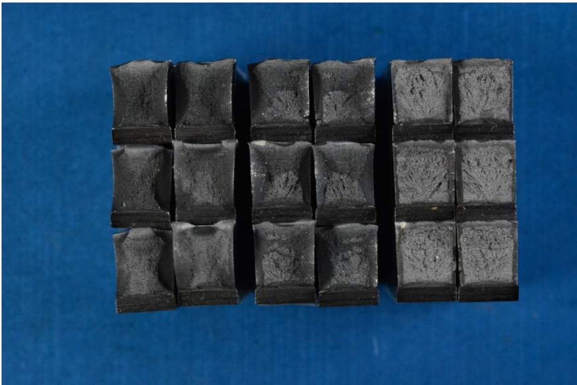
Figure J-4 - \frac{3}{4} -size Charpy fracture surfaces for Galvanized Threadbar®. From left to right, test temperature was 90°F, room temperature, and -30°F.
