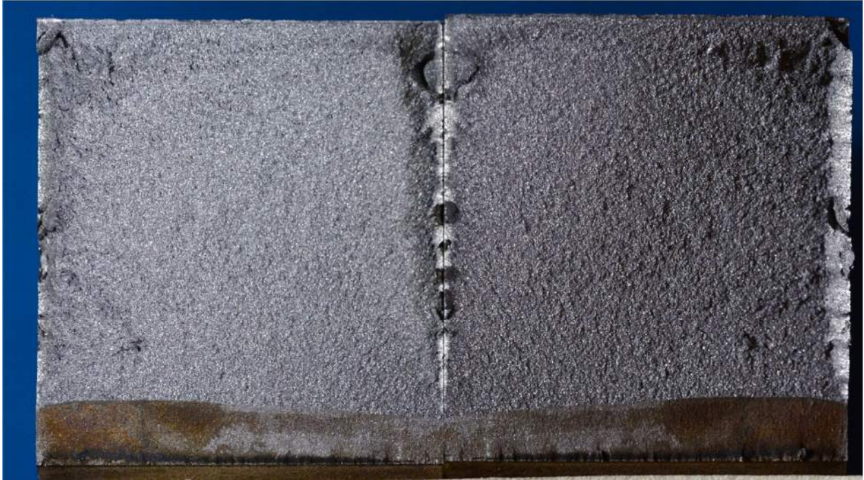
Figure N-8 – Threadbar® Plain charged RSL fracture surfaces.
