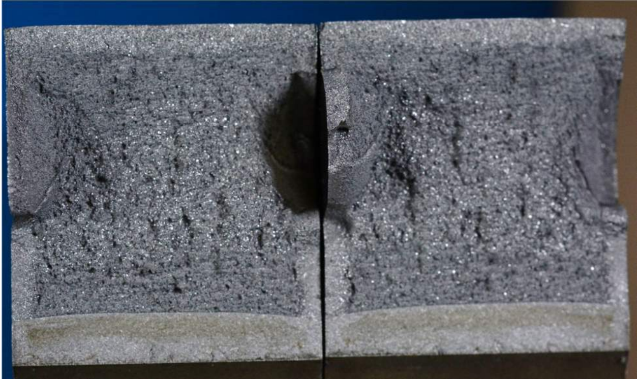
Figure N-16 – Custom 630 H1100 charged RSL fracture surface.
