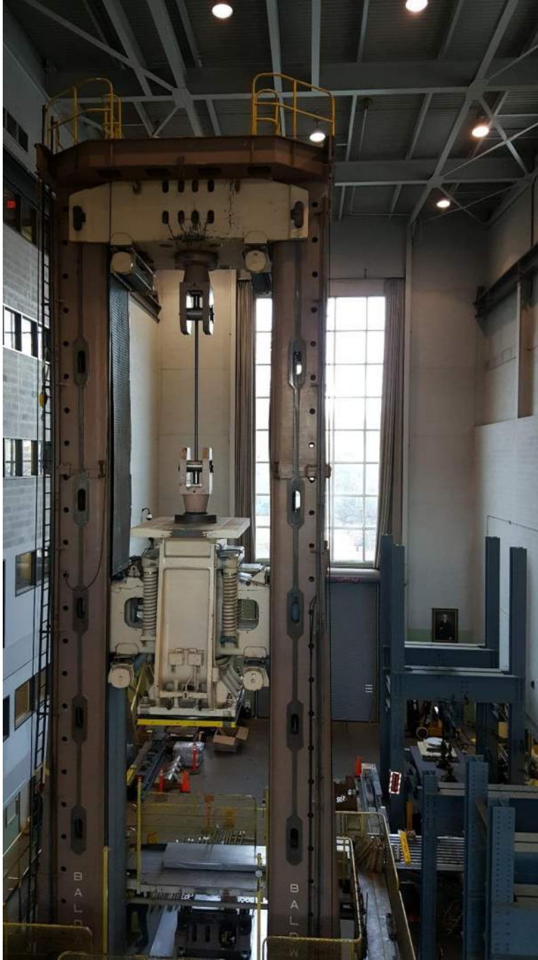
Figure 4.1-1 –Tension test setup in Universal Testing Machine (Note for scale: The test specimen is a 12 ft bar).
