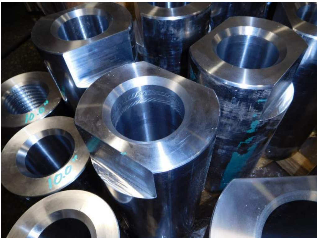
Figure D-6 – Nuts prior to internal threading.
