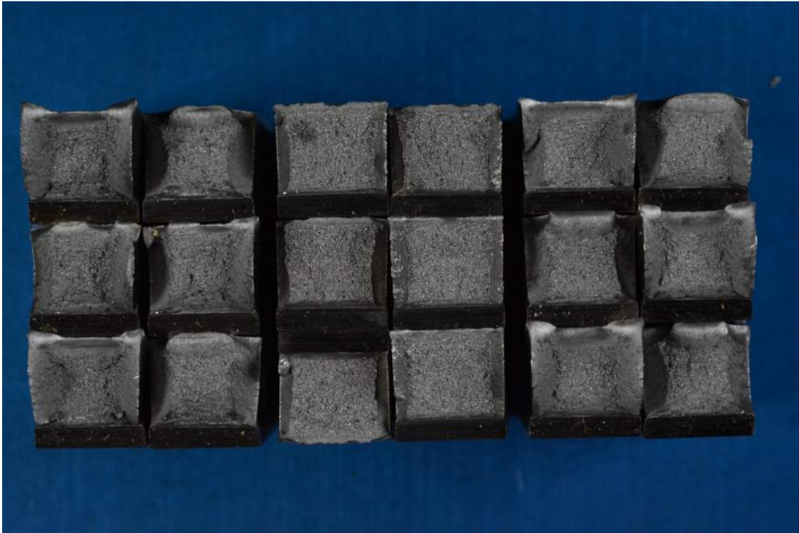
Figure J-7 - Full-Sized Charpy fracture surfaces for Custom 630 H1100. From left to right, test temperature was 90°F, room temperature, and -30°F.
