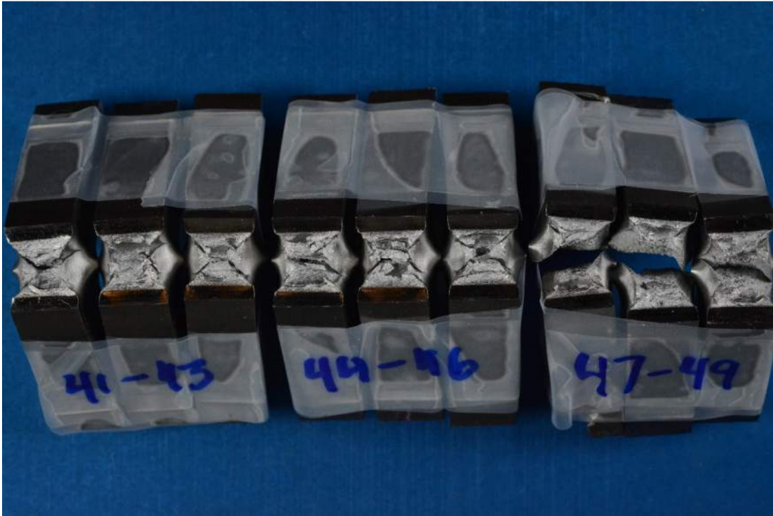
Figure J-9 - Full-Sized Charpy fracture surfaces for Alloy 2507. From left to right, test temperature was 90°F, room temperature, and -30°F.
