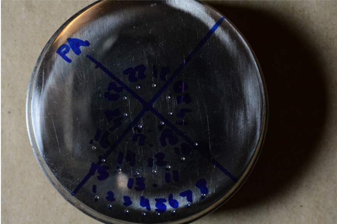
Figure H-1 - Plain Threadbar®, Rockwell C hardness measurements.
