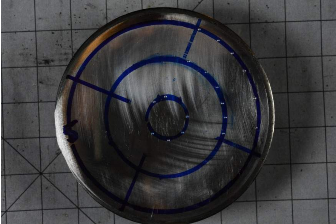
Figure H-5 - Alloy 2507, Rockwell C hardness measurements.
