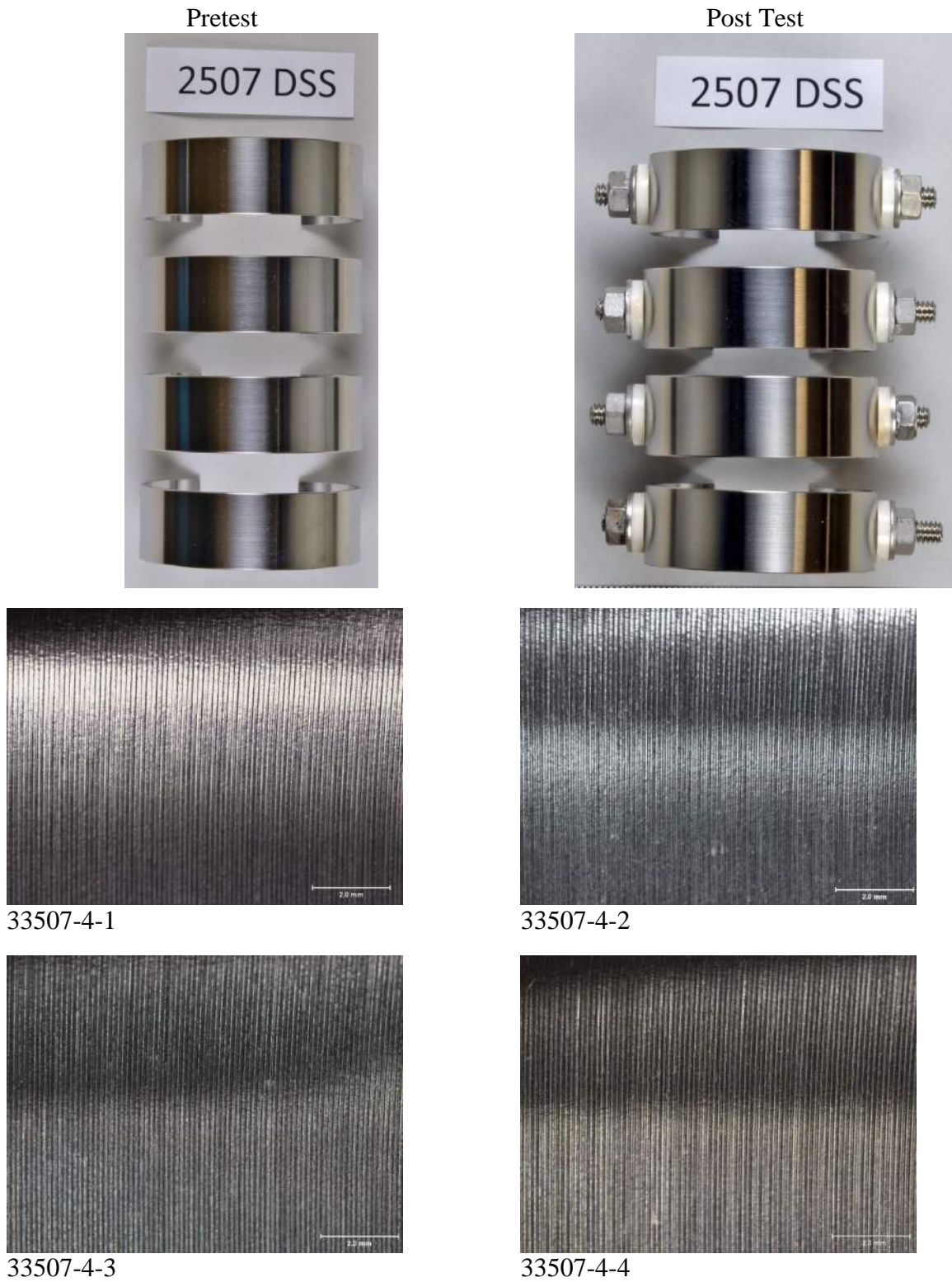
Figure 7. 2507 DSS C-rings, Top: before and after exposure; Middle and Bottom: close-up (11X original magnification) on each C-ring after exposure for 14 days per ASTM G123.
