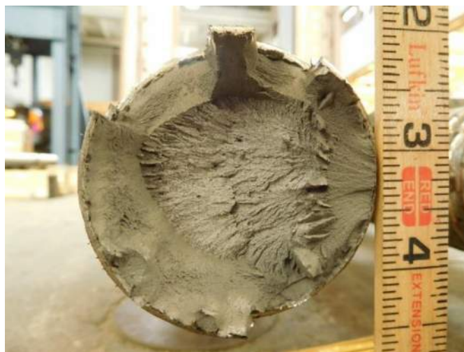
Figure 5-1 - Plain Threadbar ® fracture surfaces.
