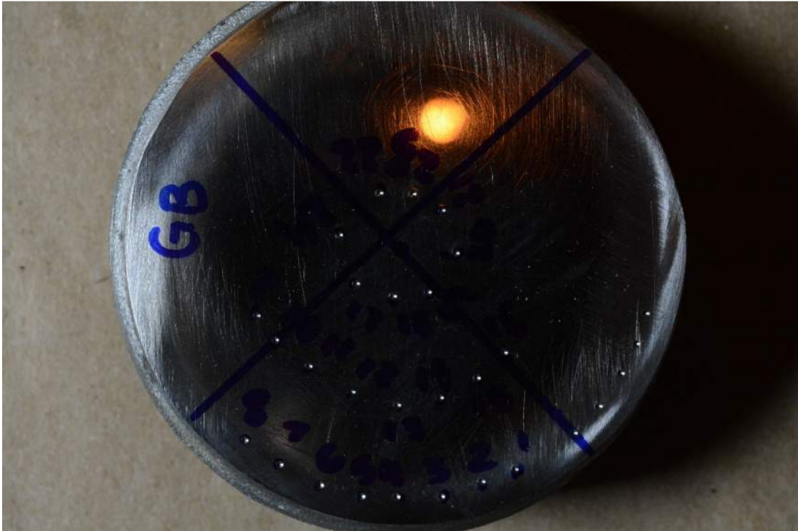
Figure H-2 - Galvanized Threadbar®, Rockwell C hardness measurements.
