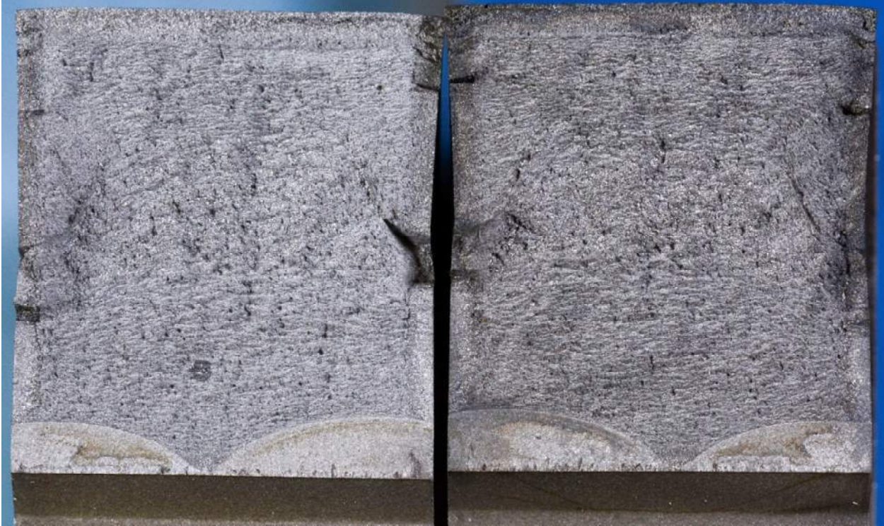
Figure N-12 – Custom 450 H1050 charged FFS fracture surfaces.
