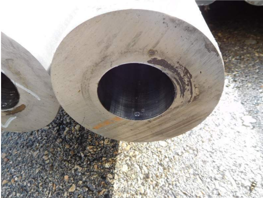
Figure D-5 – Bar stock following trepanning.
