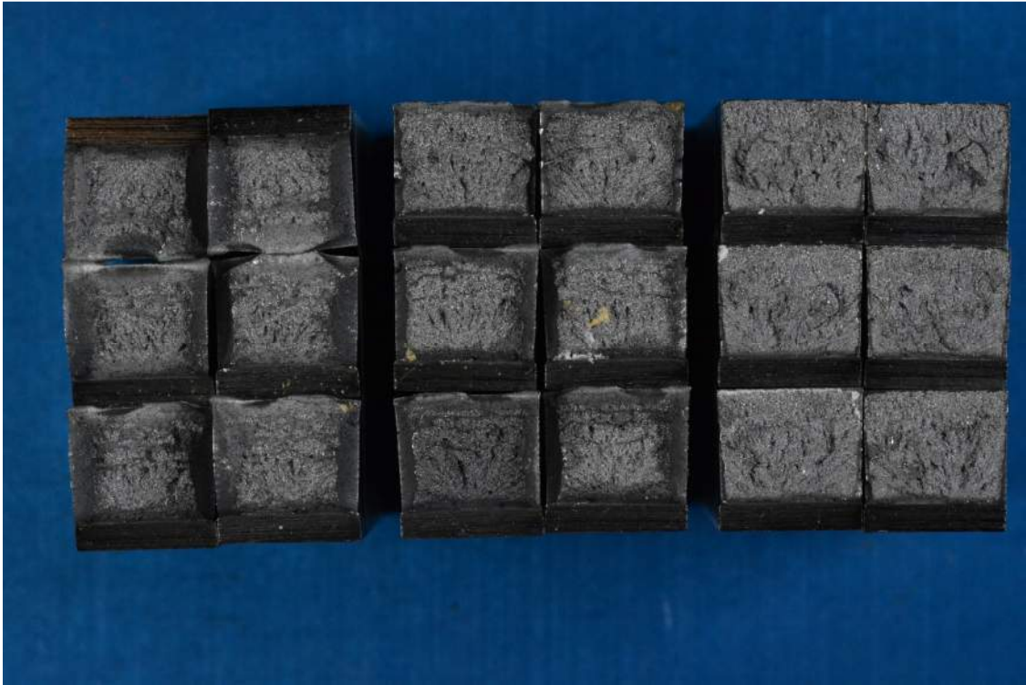
Figure J-1 - Full-Sized Charpy fracture surfaces for Plain Threadbar®. From left to right, test temperature was 90°F, room temperature, and -30°F.
