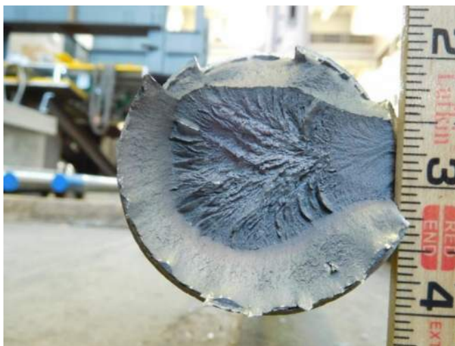
Figure 5-2 - Galvanized Threadbar ® fracture surfaces.
