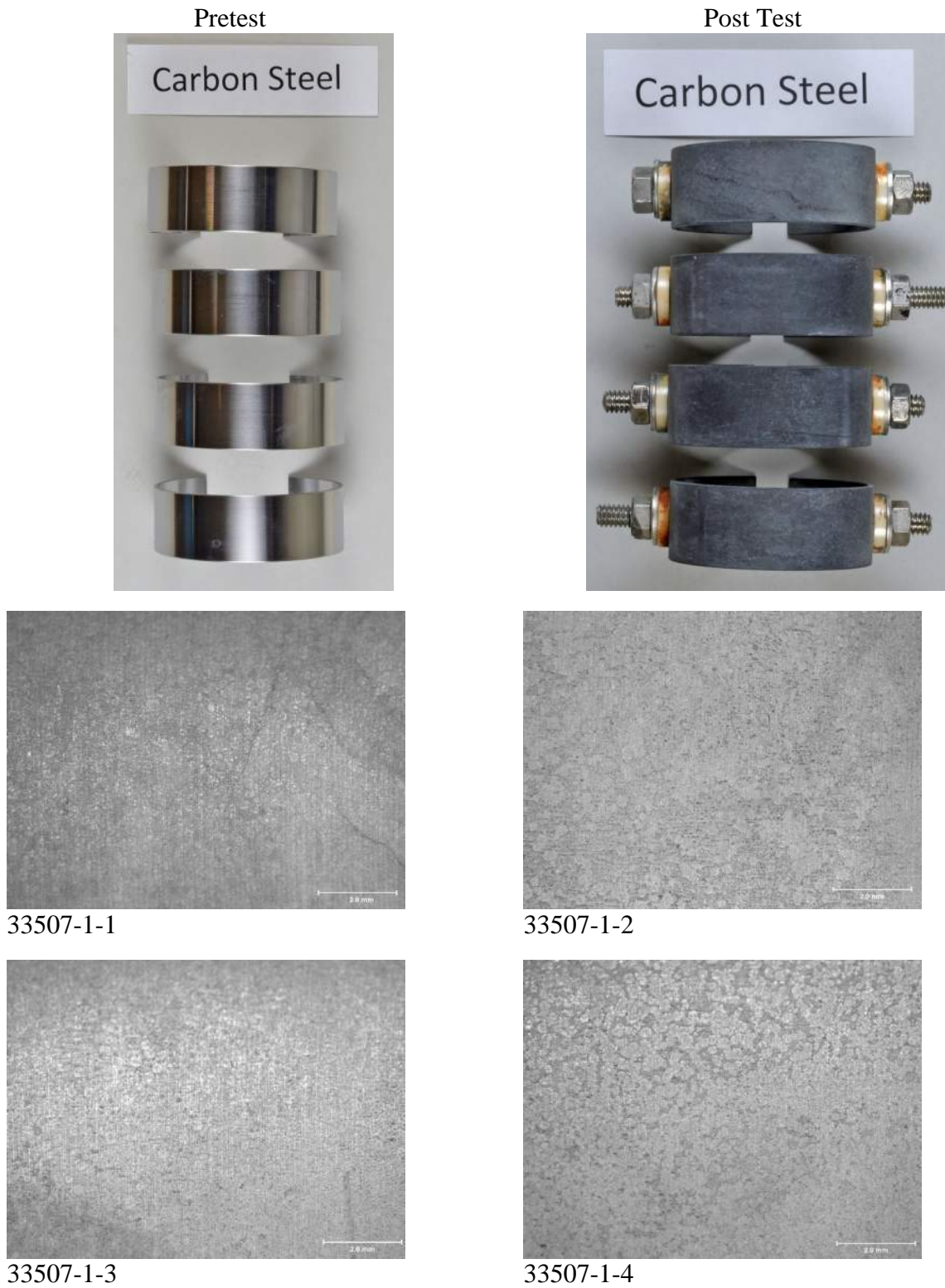
Figure 4. Carbon Steel C-rings, Top: before and after exposure; Middle and bottom: Close-up (11X original magnification) of each C-ring after exposure for 14 Days per ASTM G123.
