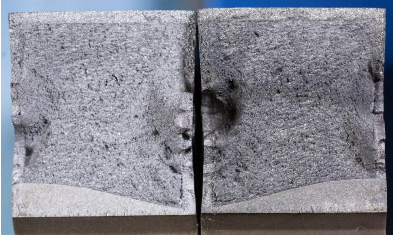
Figure N-15 – Custom 630 H1100 charged FFS fracture surfaces.
