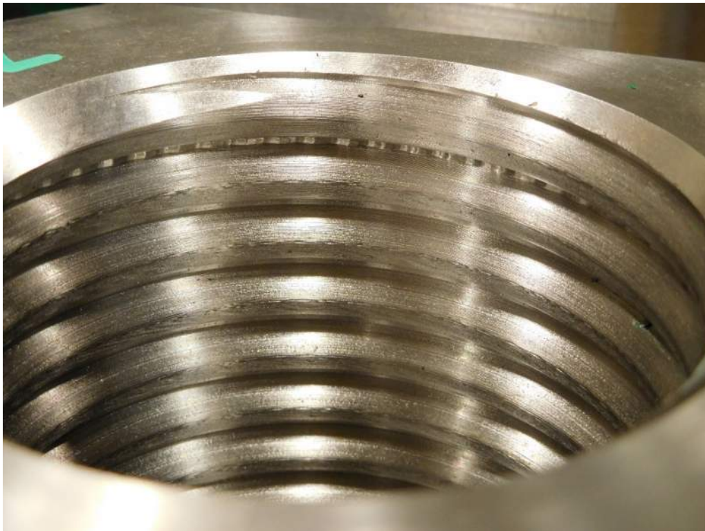
Figure D-8 – Internally threaded stainless steel nut.
