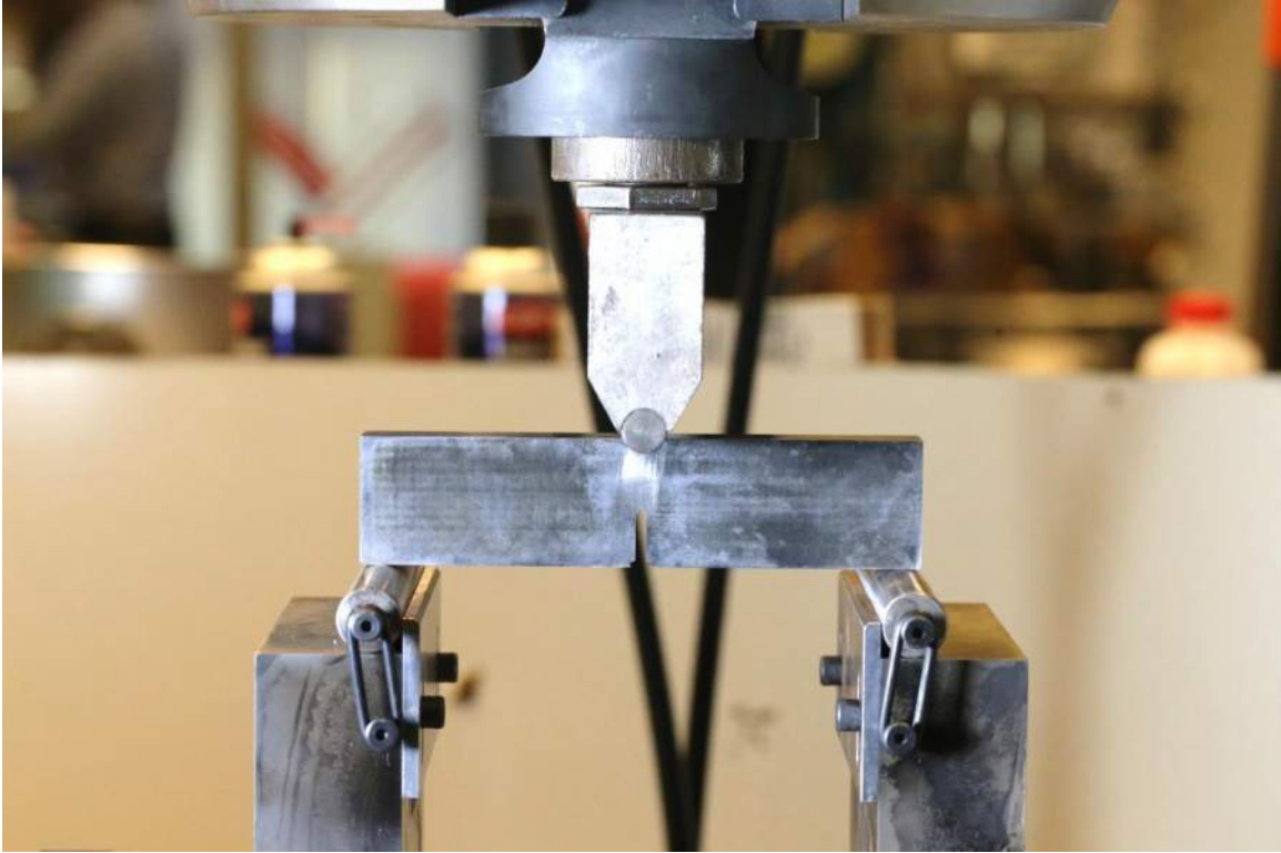
Figure 4.10-1 – Pre-cracking Test Setup.
