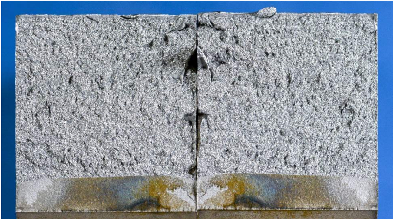
Figure N-7 – Threadbar® Plain charged FFS fracture surfaces.
