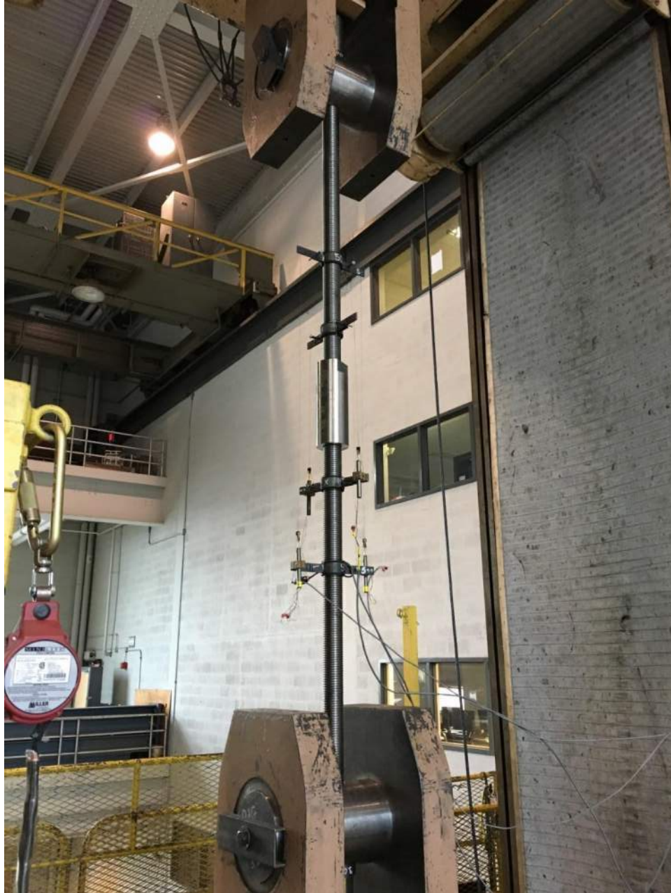
Figure 1: Typical Coupled Bar Assembly Installed in Test Machine
