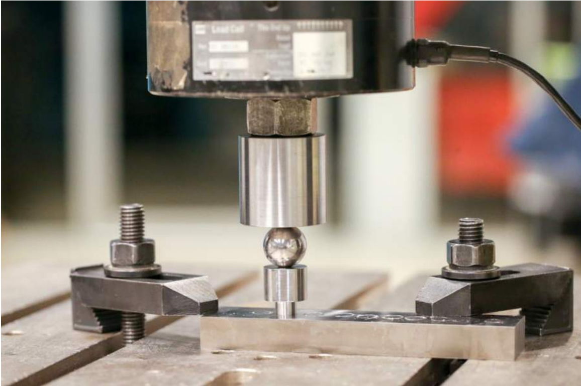
Figure 4.7-1 – Galling test setup.
