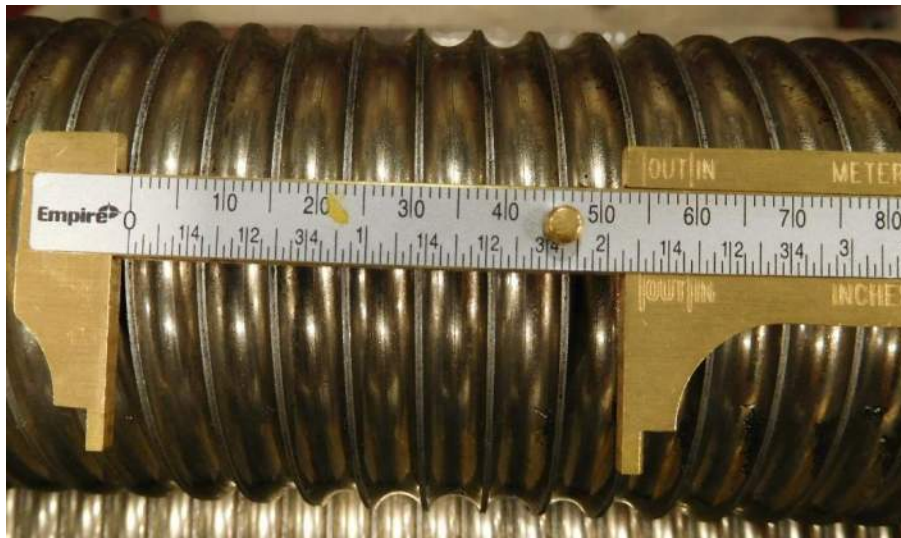
Figure 3-3 – Representative thread size and pitch of the threaded bar.
