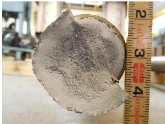
(b) End view of the fracture surface.
