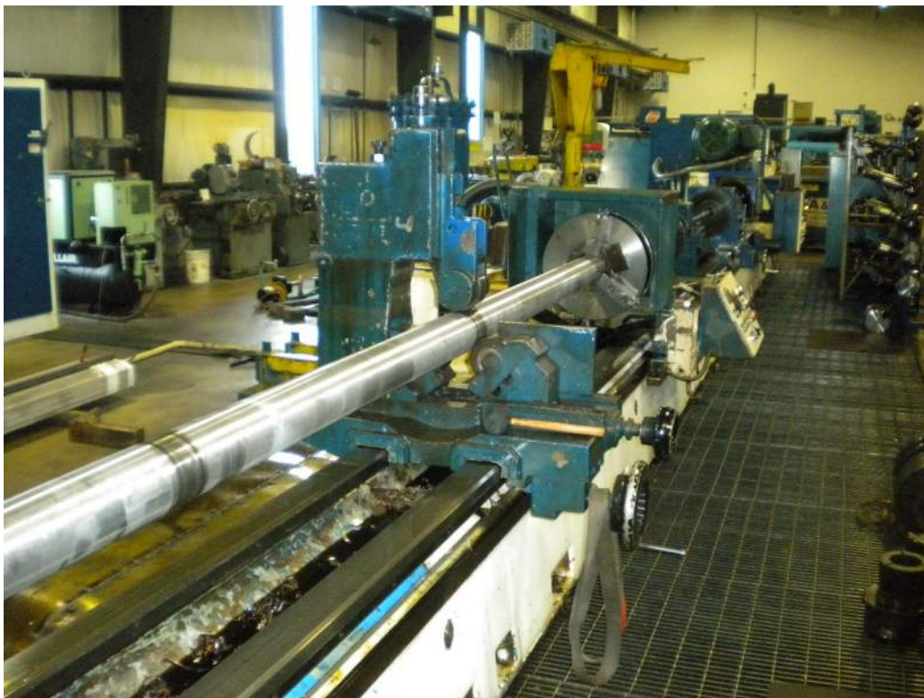
Figure D-4 – Trepanning (bar stock at near end, drill bit, and extension at far end of machine).
