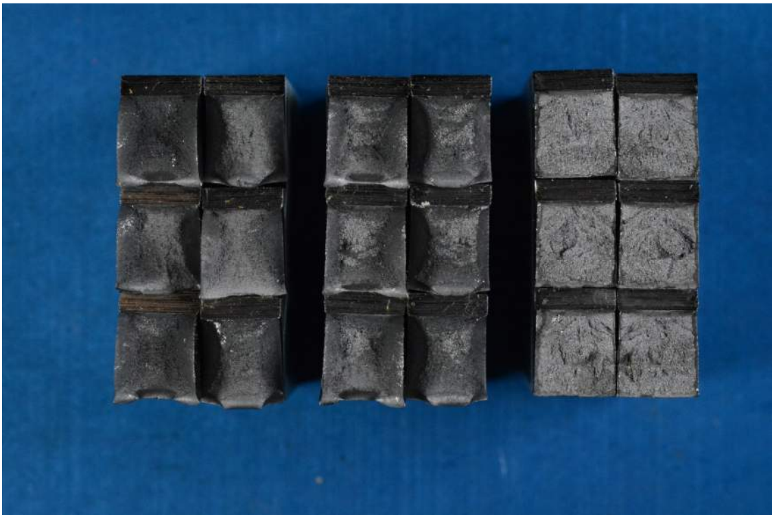
Figure J-2 - \frac{3}{4} -size Charpy fracture surfaces for Plain Threadbar®. From left to right, test temperature was 90°F, room temperature, and -30°F..
