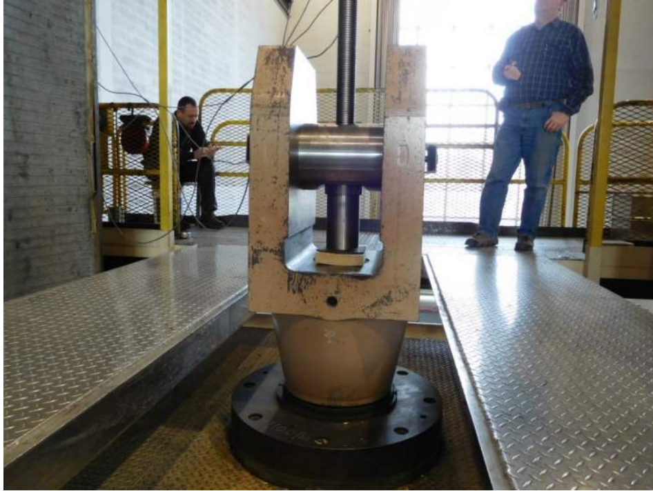
Figure E-16 – End support condition showing the end nut reacting against a clevis pin in the testing machine. (Note wood board below nut intended to absorb energy at failure and prevent damage.)
