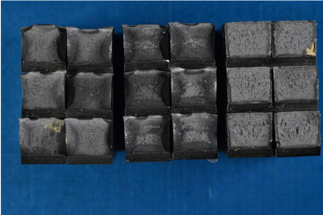
Figure J-3 - Full-Sized Charpy fracture surfaces for Galvanized Threadbar®. From left to right, test temperature was 90°F, room temperature, and -30°F.
