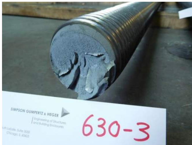
Figure 5-4 - Custom 630 stainless steel fracture surfaces.
