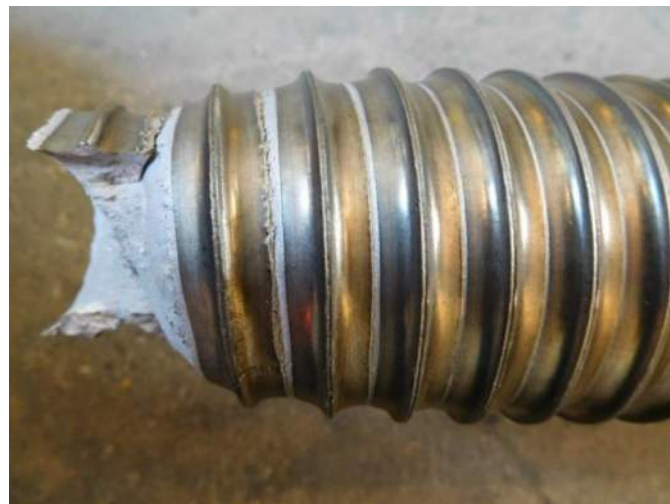
(c) Side view showing the irregular fracture surface.
