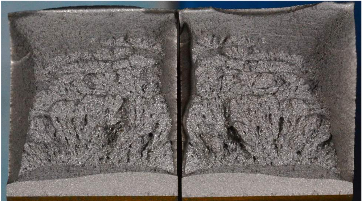
Figure N-9 – Threadbar® Galvanized uncharged FFS fracture surfaces.
