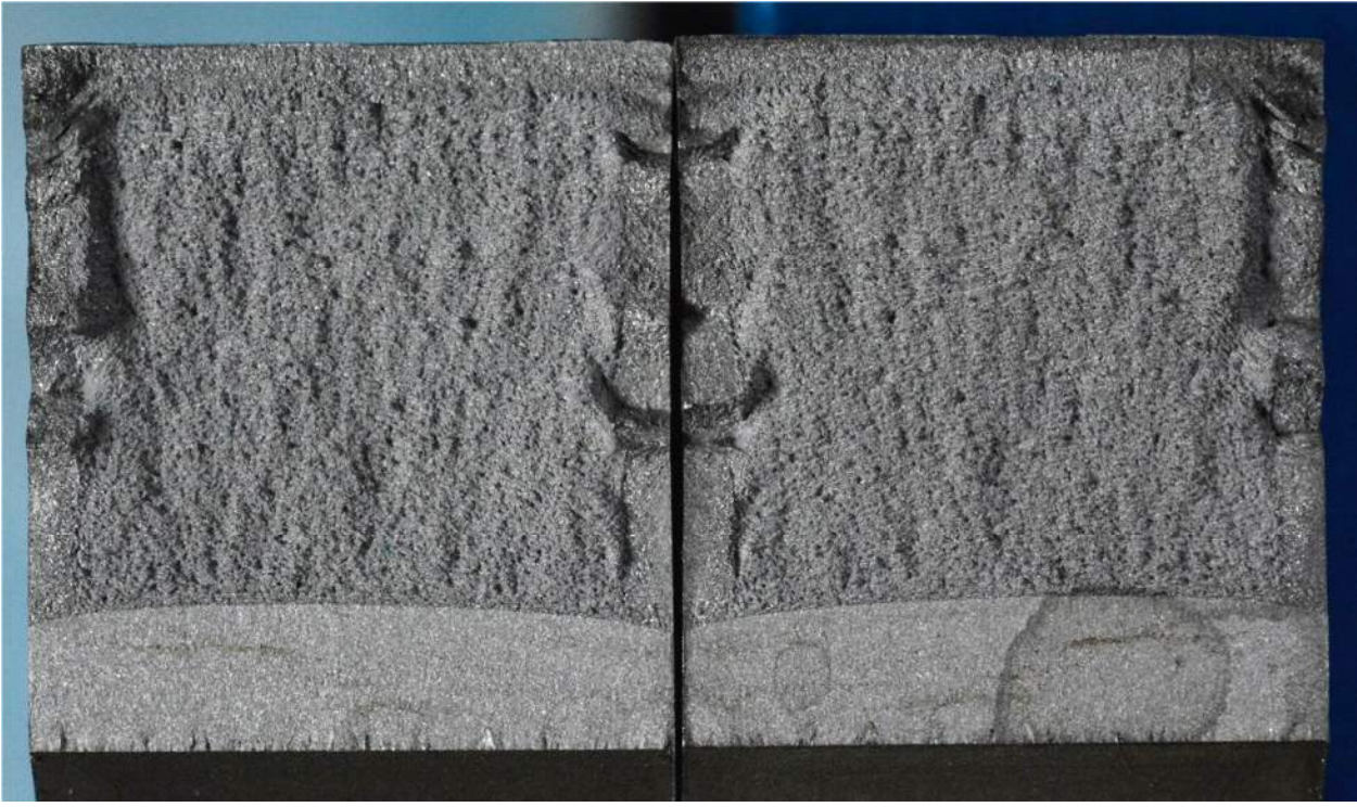
Figure N-13 – Custom 450 H1050 charged RSL fracture surfaces.
