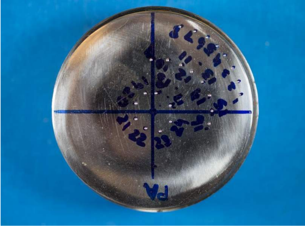
Figure 4.5-1 – Sectioned bar showing tested hardness locations (plain Threadbar® shown).
