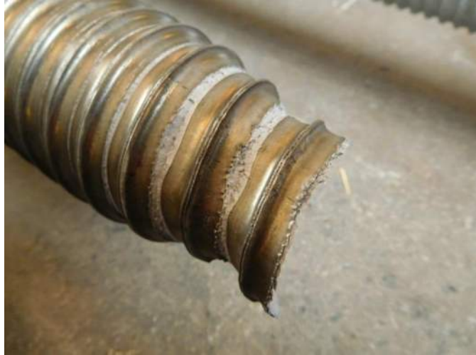
(a) End showing metal tearing in the thread roots.
