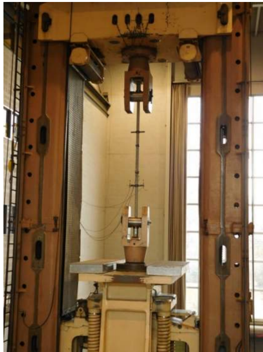
Figure E-17 – Initial tension loading up to approximately 0.9% strain showing the instrumentation set-up with extensometers at the two gage lengths measured.
